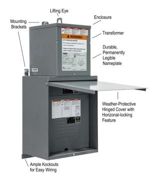
in both single- and three-phase power solutions. Housed in a NEMA 3R enclosure, it is UL Listed for both indoor and outdoor applications and is also rated for service entrance use. Both the transformer and panelboard steel enclosures are protected by an electrostatically applied powder coating for added corrosion resistance against wet, dirty, or dusty environments. Bolt-on versions of the Mini Power- Zone available in stainless steel.
